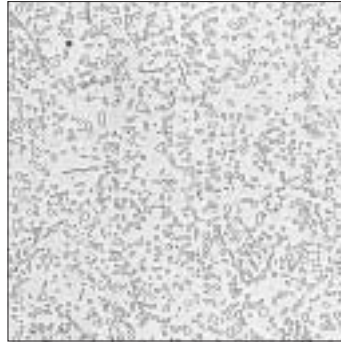
Good spheroidization Corrosion picral X400
