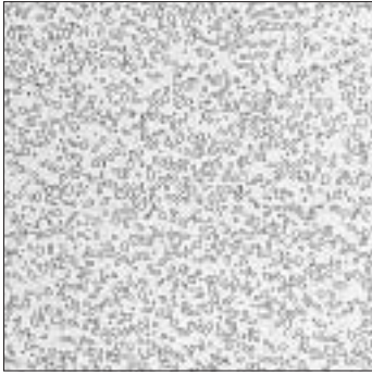
Excellent spheroidization Corrosion picral X400
